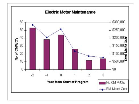
Another measure of success is the industry accepted "CBA" Cost Benefit Analysis associated with the Condition Based Maintenance Program. Below are savings calculated by the AEP CBM program over 3 years.
